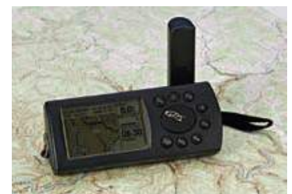
Figure 1.28 A GPS (Global Positioning System) receiver
