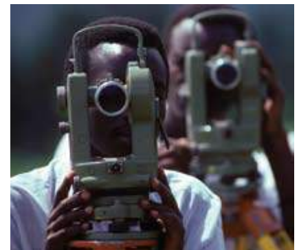
Figure 1.27 A theodolite – this is used to measure the height of trees or of slopes in the area
