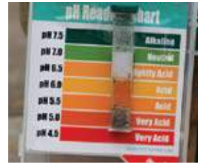
Figure 1.24 A pH kit – this is used to measure the pH of soil or water
