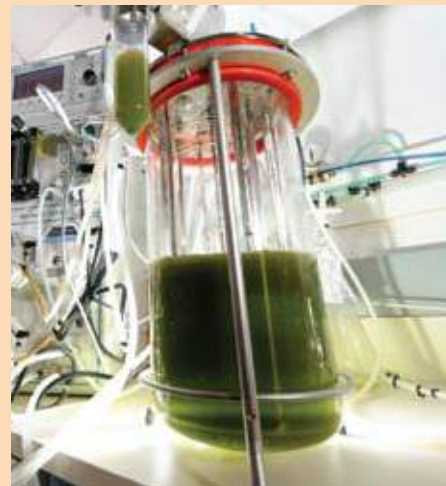
Figure 5.26 A fermenter that monitors changes electronically
