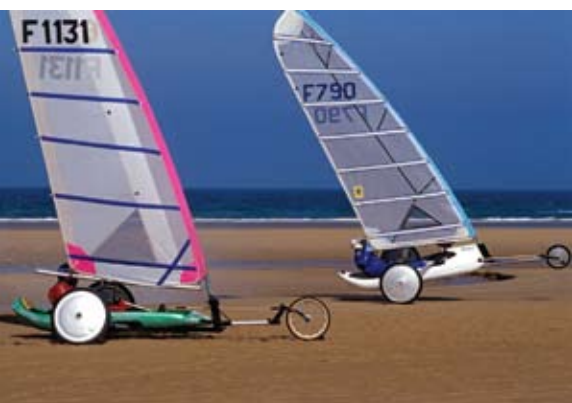
Figure 8.29 The wind passing in front of the sail is fast enough to experience a significant reduction in pressure and the sail is pulled forward
