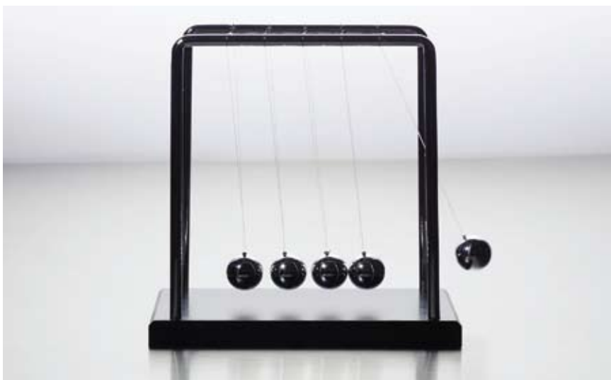
Figure 4.21 A Newton's cradle relies on the law of conservation of linear momentum to work.
