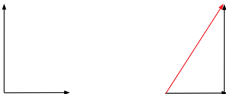
Figure 2.20 Two perpendicular coplanar vectors
